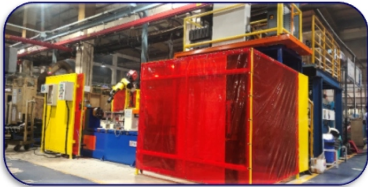
VP SYNERGIC ROBOTIC HYDRAULIC CYLINDER BARREL TO END CAP, BRACKET, PORT & PISTON ROD TO ROD EYE WELDING SPM
