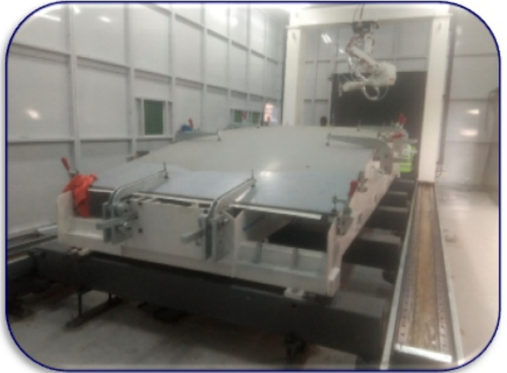
VP SYNERGIC ROBOTIC HYDRAULIC CYLINDER BARREL TO END CAP, BRACKET, PORT & PISTON ROD TO ROD EYE WELDING SPM
